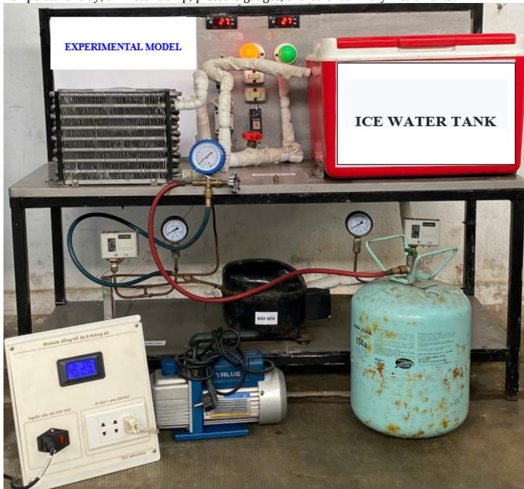
Figure 5: Experimental model of the refrigeration system equipped with a heat recovery device
