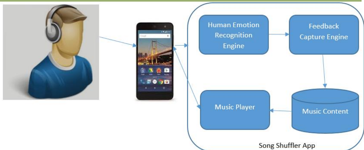
Fig 2: Quick View of the Key Components of Song Shuffler
