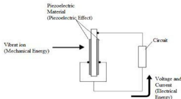
Fig1.schematic of a piezoelectric damper.
