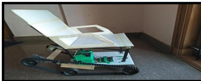
Fig. 9 assembly of stair climbing wheel chair
