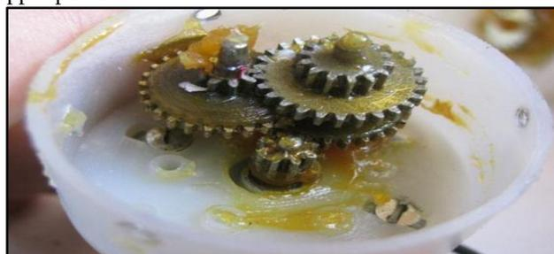
**Fig. 3** internal structure of geared dc motor
