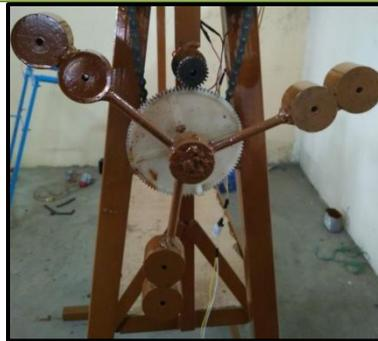
Fig. 7 spur gear assembly
