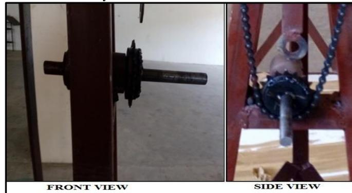
Fig. 5 two views of free wheel assembly
