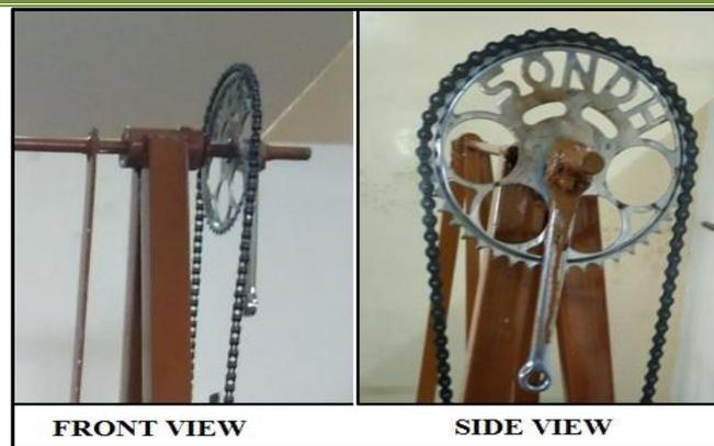
Fig. 4 two views of sprocket assembly
