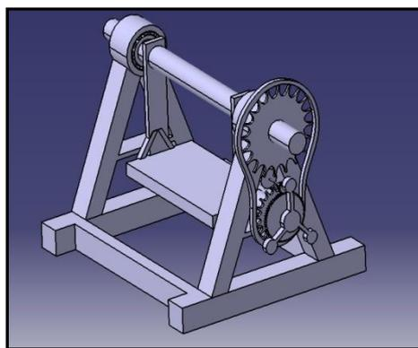
Fig. 3 3-D model of swing motion power generation
