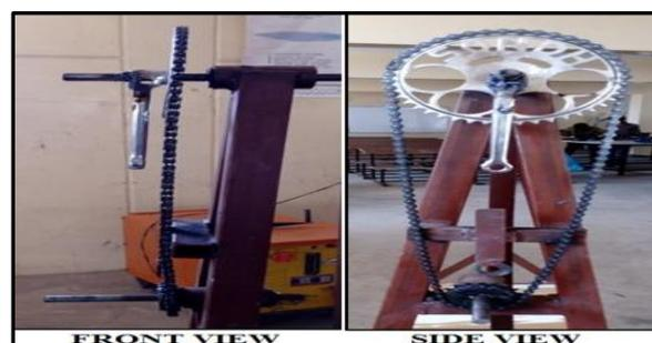
Fig. 6 two views of chain drive assembly
