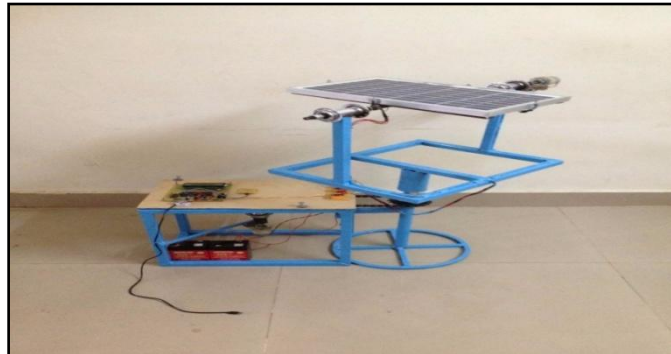
Fig. 5 assembled model of the coin based cell phone charger by usin solar tracking system
