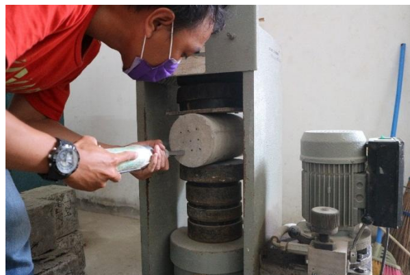
Figure 5. Test the hammer on a concrete cylinder
