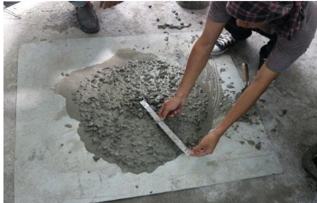
Figure 3. Results of slump flow spread test
