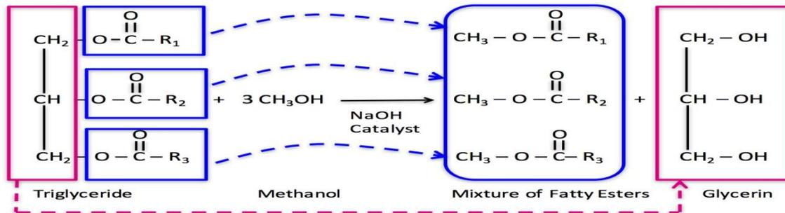
Figure 1; Transesterification chemical equation [9]
