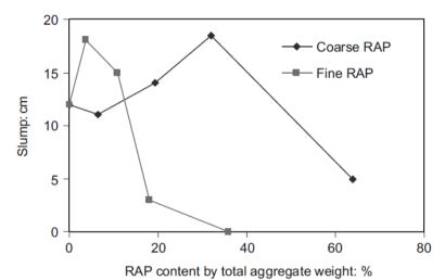
Fig. 2 Relation between slump and RAP content. [5]
