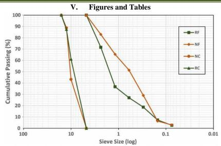
Fig.1 Grain size analysis of natural and RAP aggregates [31]
