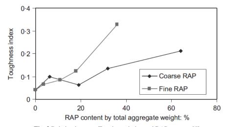
Fig. 3 Relation between Toughness index and RAP content. [5]
