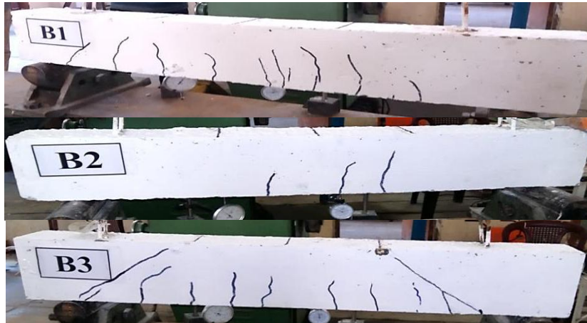
Fig.5 Failure mode and crack patterns of tested beams
